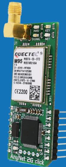
The new AnyNet Click can easily be deployed on any MikroElektronika development board, or any board that hosts a mikroBUS™ socket, and tested in multiple combinations across the full range of microcontroller and click boards. It gives developers throughout the world the freedom to rapidly build IoT devices and is the ideal platform on which to develop and test M2M IoT, and to utilise AWS Cloud data analytics tools.
